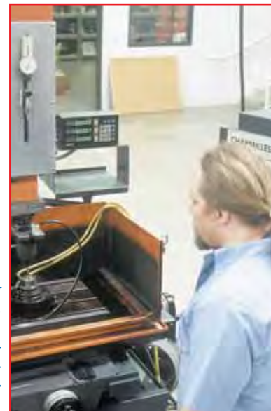
Contemporary EDM technology is used to perform special operations, such as hex-broaching the nose of a unique short-run fastener
