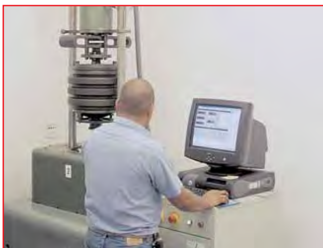
ARP has two of these highly sophisticated Amsler fatigue machines, which check fasteners through millions of cycles.
