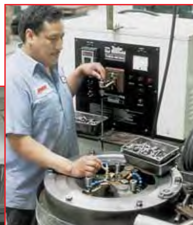
ARP performs the thread rolling operation after heat-treating, which results in a fatigue strength up to 10-times higher than fasteners with threads rolled prior to elevating the material's tensile strength.
