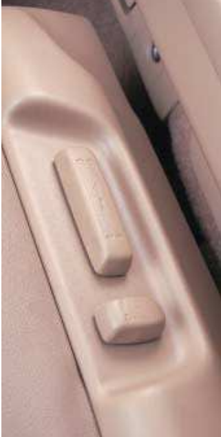
Executive models feature electric driver seat controls, with effortless eight way adjustment including 40mm of height and 80mm fore-and-aft.
